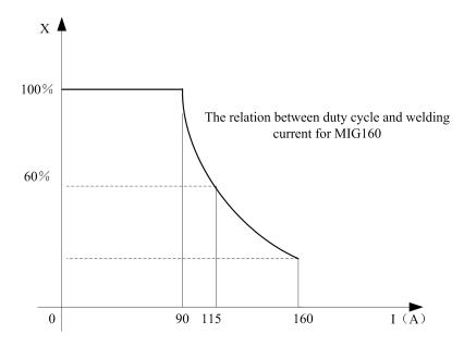
If transformer is over-heat, the heat relay inside it will open and will output an instruction to circuit board, cut AC relay and the output welding current, and brighten the over-heat pilot lamp in the front panel. At this time, the machine should be relaxed for 15 minutes to cool the fan. When operating the machine again, the welding output current or the duty cycle should be reduced.
